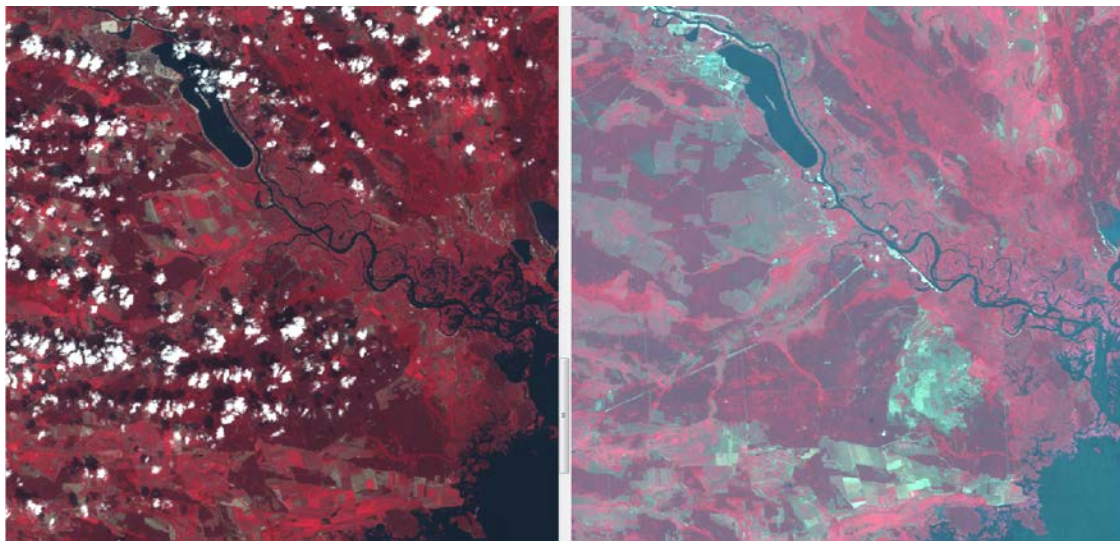
Figure 2 subset false color (1-4-7) Landsat 4 TM from 1985 and Landsat 7 ETM+ from 2001 covers study area which less covered by cloud.
